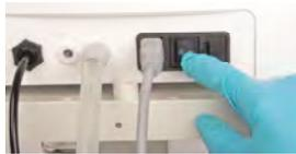
Use the power switch "I/O", at the rear of the device, to switch the device on and off. The standby is signaled by the LED status light at front of the device. The device can be switched off at any time, irrespective of any procedure for device switch-off.
