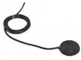
The included standard pneumatic ON/OFF-pedal when pushed activates a switch in the Vacuson pump, to switch the pump on and off. This is maintained by an air pillow. After the device was switched on, the pneumatic pedal has to be pressed to activate the pump and generate vacuum. Pressed again the pump is deactivated. The pump can only be activated by the pedal. The last used state before switch-off stays active.
