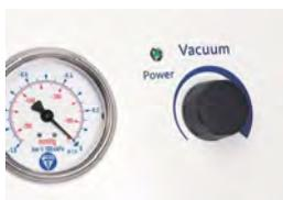
The suction process is regulated by the Vacuum controller at the front side of the device.
