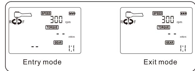
③ Auto reverse mode: when press the MODE key unit enter this mode, file can forward and reverse automatically refer on the torque, Press MODE key again, unit will exit this mode;
