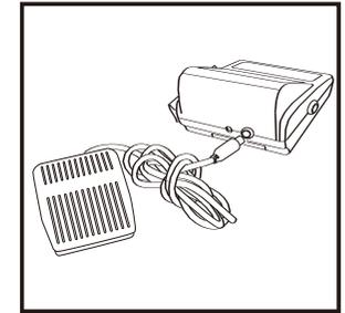
2. Insert the foot switch plug into the jack on the main unit.
