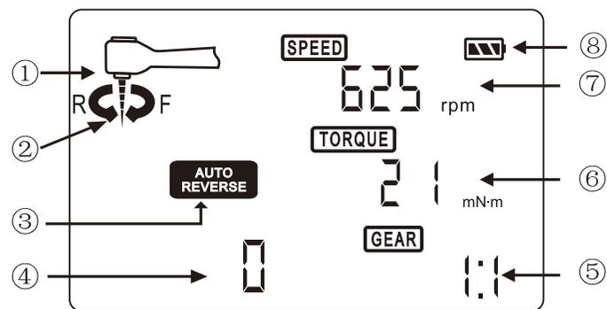
① Rotation direction sign: display **F** for forward and **R** for reverse;
