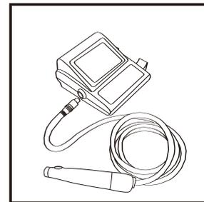
3. Connect the plug of the motor or wire to the main unit, make sure that they are in the right position.
