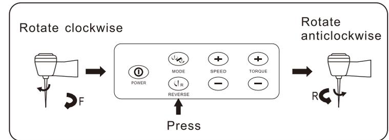
\* You can adjust speed by press "SPEED+" or "SPEED-" button when endo motor is working.
