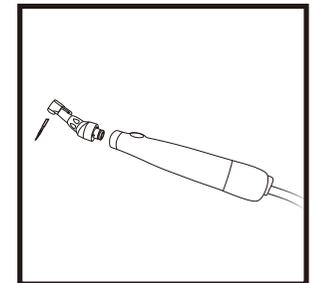
4. Connect the contra angle to the motor and clamp the file into the contra angle.
