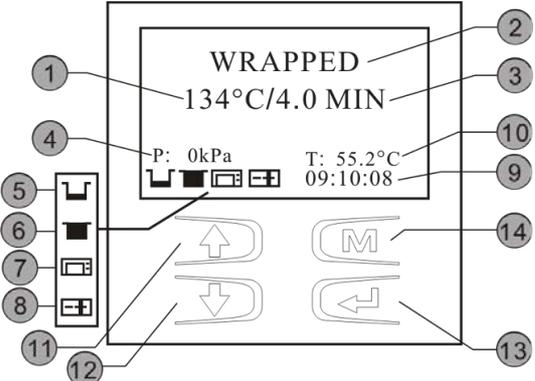
The control panel displays the following information and controls:
