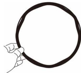
Press the remaining sections of the seal.
