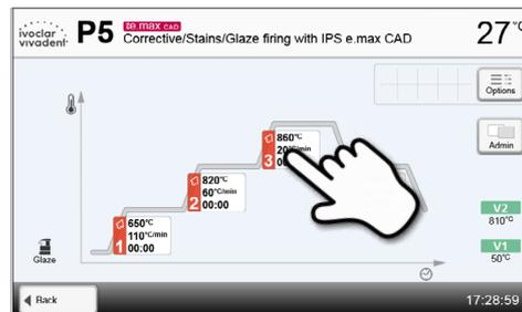
In the parameter view, the parameters can be changed. Up to three heating (a) and two cooling (b) stages are available.
