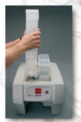
1) The access to the tank is immediate, and you can dismount it in a few seconds. You can load the tank from any comfortable position, without having to lift heavy bags over the machine. Besides, it prevents the powder generated during the operation to settle on the machine. Another advantage is the easy cleaning of the dosage system.
