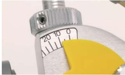
Bennett angulation indicator and setting mechanism
