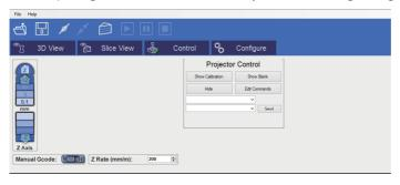
From this screen we will be able to control the motors of the printer, which means displacing the build base over the Z axis, as well as controlling the LCD.
