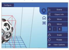
The Mirror view allows you to mirror the selected object on the specified axis.
