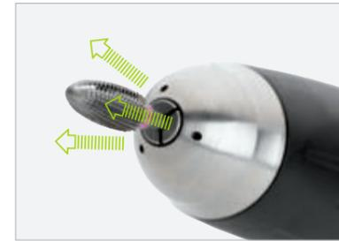
The integrated air-jet function simply blows chips and dust away. It also cleans the chucking system at the same time.
